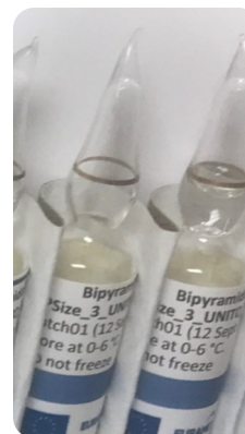
Ampoules with the 2 mL liquid suspension of bipyramidal TiO 2 nanoparticles and electron micrographs (SEM and STEM-in-SEM) with the particles deposited on a carbon TEM grid according to the protocol.
