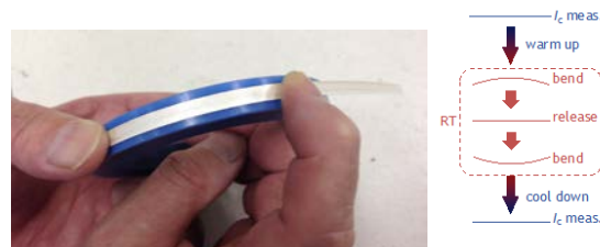
Figure 1. Double bending at room temperature for Bi-based high temperature superconducting wire
