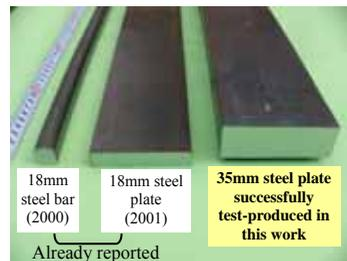
Fig.2 Appearance of test-produced large-scale UFG plate.
