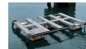
The performance of marine paints is evaluated by submerging test plates coated with the paints in seawater. The plates are inspected weekly to determine the extent to which marine organisms have attached to their surfaces.
