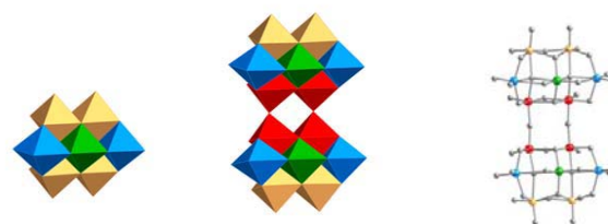
Fig. 2. (a) Schematic diagram of generation of [(\text{MoVI } 6 \text{ MoVO}_{23})_2]_{10-} from [\text{MoVI}_7 \text{ O}_{24}]_6- by a two-electron photoredox reaction. (b) Atom-and-bond representation of [(\text{MoVI}_6 \text{ MoVO}_{23})_2]_{10-} . (\text{MoVI}(1), \text{MoVI}(1)\text{O}_6 \text{ octahedra}), (\text{MoVI}(2), \text{MoVI}(2)\text{O}_6), (\text{MoVI}(3), \text{MoVI}(3)\text{O}_6) and (\text{MoV, VI}(4), \text{MoV, VI}(4)\text{O}_6) are indicated by yellow, blue, green and red, respectively. four \text{MoV, VI}(4)\text{O}_6 octahedra (Fig. 2(b)) [41]. In the present work, we measured ^{95}\text{Mo} solid-state magic-angle-spinning (MAS) NMR spectra of 1 and 2 under moderate (9.4 T) and ultrahigh fields (21.8 T). By simulating the acquired spectra, contributions from chemical shift and quadrupole interactions were extracted separately. Origin of large chemical shift for MoV or MoV, VI species was briefly discussed
