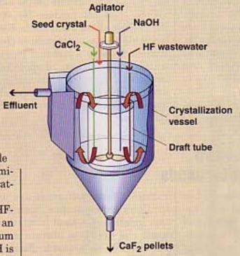
scales, and limited to HF concentrations below 1%, says the firm. Organo plans to market CaF2-recovery plants to match customer's requirements, and says the technology is suitable for other industries besides semiconductor manufacturing that use HF, such as glass making and fluorochemicals production. Plants treating 6-100 m3/d of wastewater containing 1-9% HF will have CaF2-production capacities of 300 to 5,000 kg/d, says the firm.
