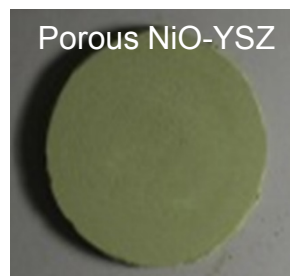
Anode-supported SOFC (GDC/LSGM/GDC layered composite)
