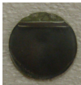
Anode-supported SOFC (GDC/LSGM/GDC layered composite)
