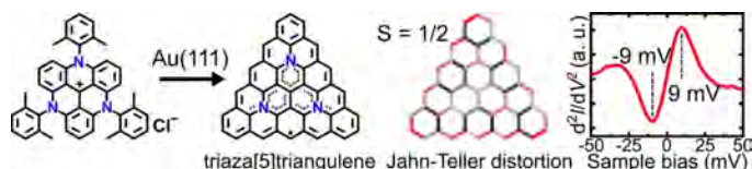
Figure: Triaza[5]triangulene, containing three graphitic nitrogen atoms synthesized on Au(111) through cyclodehydrogenation.
