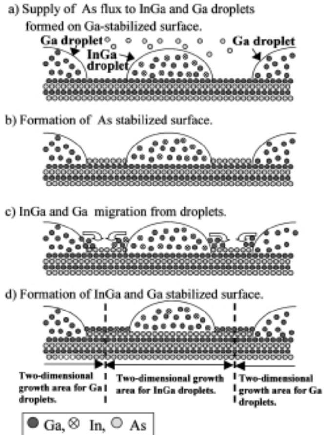
Fig. 2. The schematic model of InGa and Ga droplets during As molecular beam supply for crystallization.
