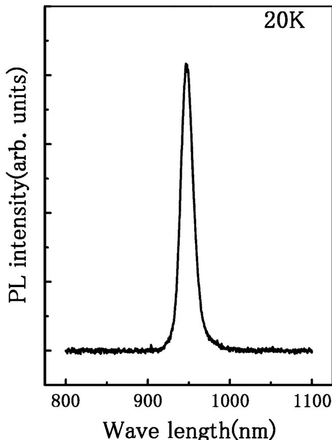
Fig. 4. Photoluminescence spectrum for capped InGaAs QDs at 20 K.
