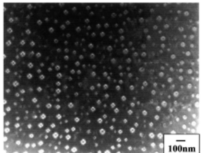
Fig. 3. Plan-view TEM image of InGaAs QDs after the crystallization and annealing process.
