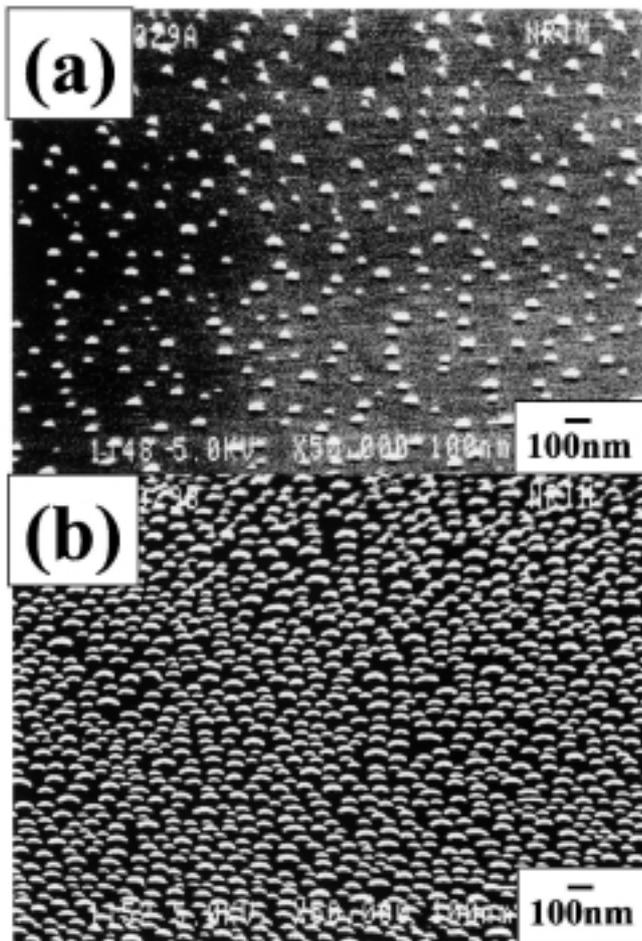
Fig. 1. HR-SEM image of droplets (a) before and (b) after the supply of 50 ML of Ga.
