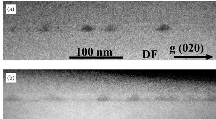
Fig. 3. Cross-section TEM images, taken along the [0 2 0] axis: (a) sample A: QDs without WL; and (b) sample B: QD with 3 MLs WL.
