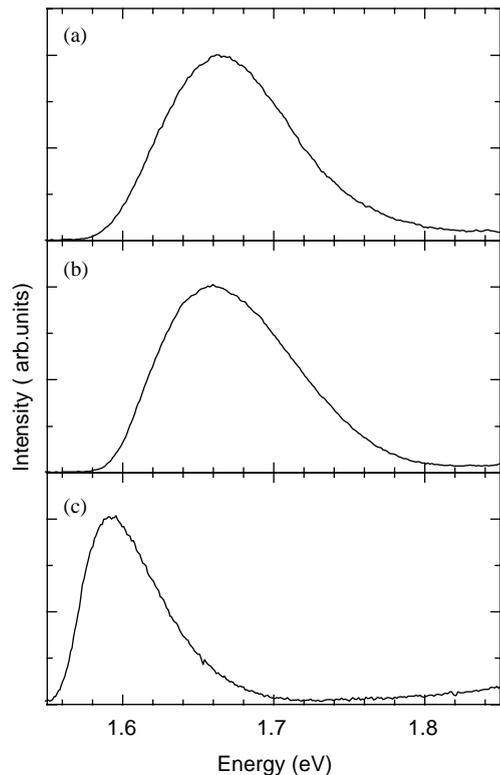
Fig. 4. Low temperature (20 K) PL spectra of the samples A (a), B (b) and C (c). The excitation power density was 5 W/cm<sup>2</sup>.
