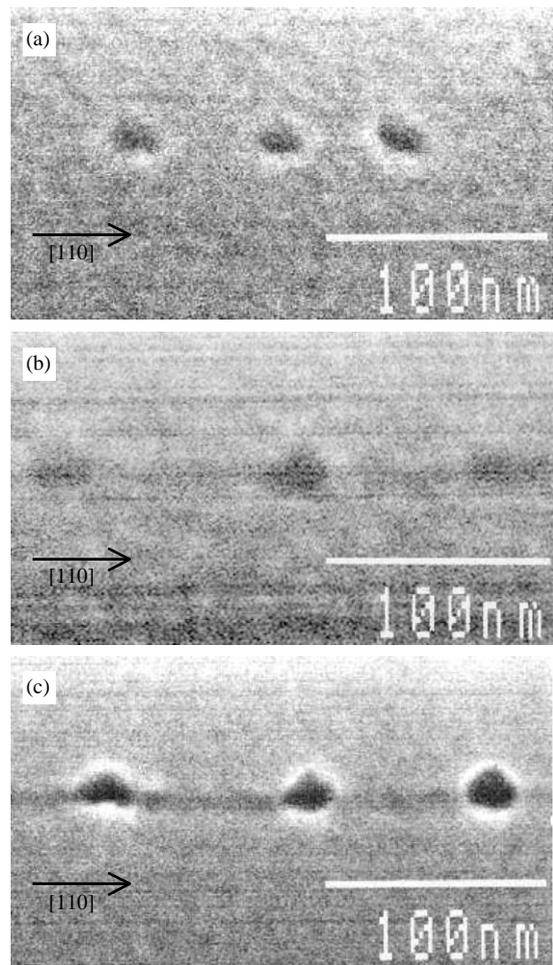
Fig. 2. Cross-section TEM micrographs, taken along the [110] axis: (a) QDs without WL; (b) QDs with 3 MLs WL; and (c) QDs with 8 MLs WL. In such bright-field images QD as well as the WL appear with a darker contrast.
