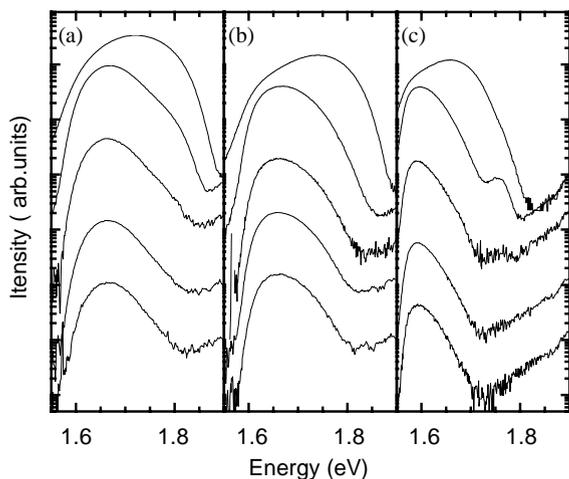
Fig. 5. Five different PL spectra taken at increasing excitation power densities at steps of one optical density in the range  $0.5 \text{ W/cm}^2$ – $5 \text{ kW/cm}^2$  of the samples A (a), B (b) and C (c). All the measurements were performed at  $T = 20 \text{ K}$ .
