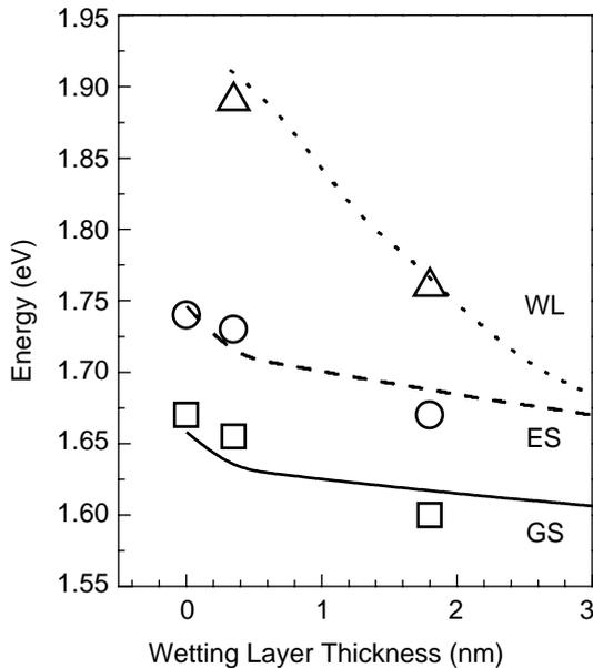
Fig. 6. Comparison between experimental and calculated transition energies of the wetting layer (triangles and dotted line) and the ground state (squares and continuous line) and the excited state (circles and dashed lines) of the QD.
