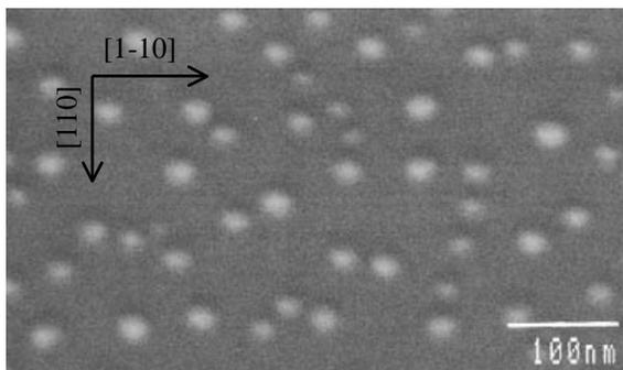
Fig. 1. Surface HREM image of an uncapped QD sample.
