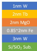
Fig. 1. Schematic of sample structures of W(3nm)/Fe(0.85-2nm)/MgO(2nm)/Tb(2nm)/W(1nm) on Si/SiO 2 Sub.
