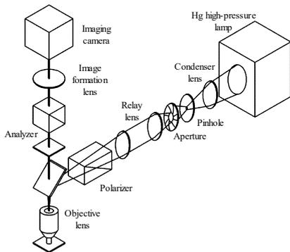
Fig. 1 Schematic of the domain observation microscope.
