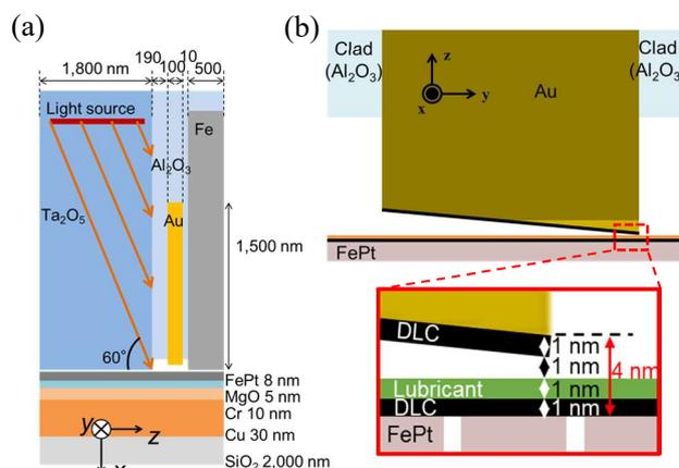
Fig. 1 The structure of HAMR head when covering a DLC and a lubricant for thermal calculation. Side view (a), NFT enlarged view (b).
