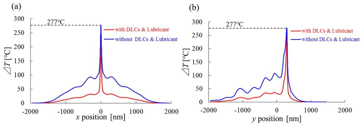
Fig. 3 Temperature distributions in the FePt recording medium along to a cross truck direction (a) and down truck direction (b) with and without the protection layers.
