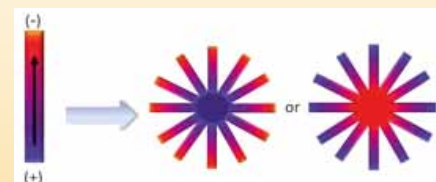
Figure 2: Schematic describing the new rule of assembly. A ZnO rod has a positive and a negative polar end, depicted in blue and red colors. Within an assembly, unipolar growth is maintained, i. e. the colors are arranged systematically, without intermixing.
