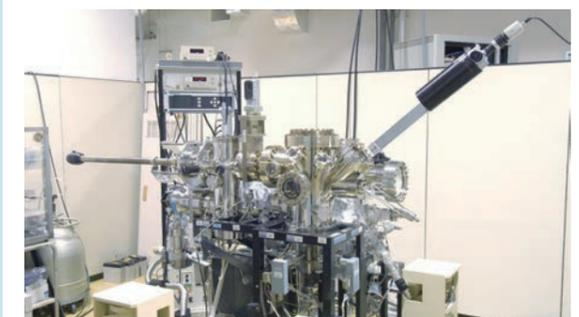
Fig. 1: The world-first double-probe scanning tunnelling microscope further improved at MANA.
