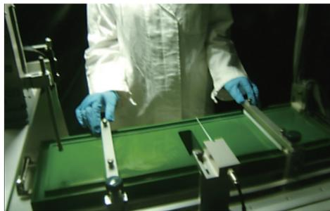
Fig. 4 Mechanism of the supramolecular system for grasping molecules with the human hand. When a supramolecular thin film on the surface of water is made to contract or expand by the movement of the human hand in our human world, corresponding to this, the molecular machine captures or releases a target molecule in the nano world.
