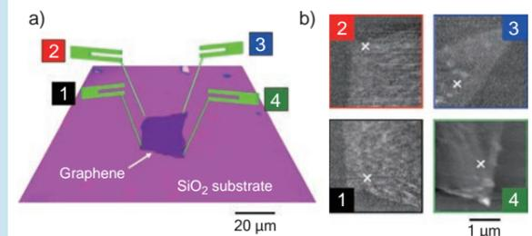
Fig. 2: Schematic diagram of a quadruple-probe atomic force microscope with tuning fork probes (TFP) enabling measurement of the properties of graphene with nanoscale precision. a) Schematic diagram of the four TFPs approaching a monolayer graphene flake measured by QP-AFM. The middle part shows the graphene flake, which is laid on a SiO<sub>2</sub> substrate. b) AFM images (3 × 3 μm<sup>2</sup> each) obtained at each corner of the graphene by using the four TFPs.
