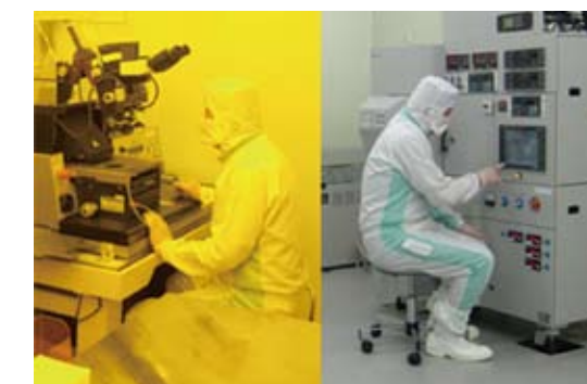
MANA Foundry Both sides mask aligner (left), Sputtering machine (right)
