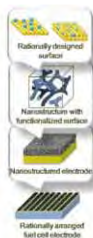
Fig. 1. Scheme for rational design of catalytic electrodes for advanced fuel cell systems by using microfabrication techniques.
