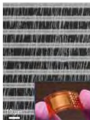
Fig. 2. SEM image of ZnO nanowire arrays bonded by Au electrodes. Inset: demonstration of an as-fabricated nanogenerator. The arrowhead indicates the effective working area of the nanogenerator.
