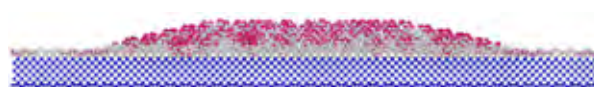
Fig. 2. Side view of a germanium nanocluster on silicon (Ge in grey, Si in blue) showing the charge density (pink) for the states near the Fermi level. 4) The model contains 23,737 atoms.
