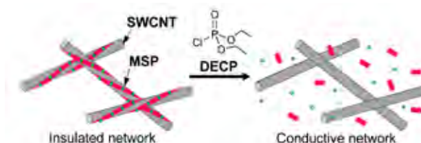
Fig. 2. Schematic illustration of chemiresistive sensor composed of SWCNTs and MSP.
