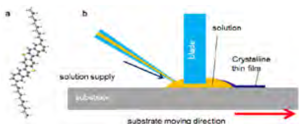
Fig. 1. Molecular structure of C_n -DNBDT (a) and the method of crystallization (b).
