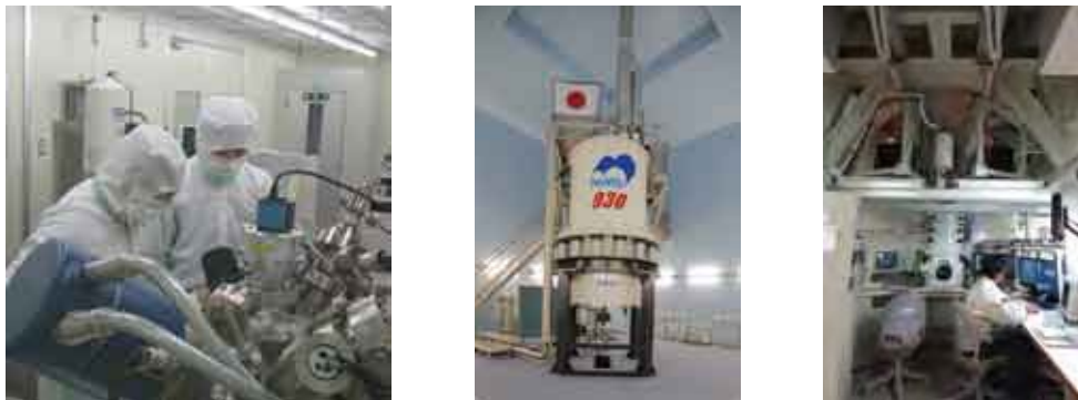
Fig. 4-4: Cutting-edge research facilities at MANA and NIMS: X-ray photoelectron spectroscopy XPS in the MANA Foundry (left), 930 MHz NMR magnet (middle) and Transmission Electron Microscope (right).
