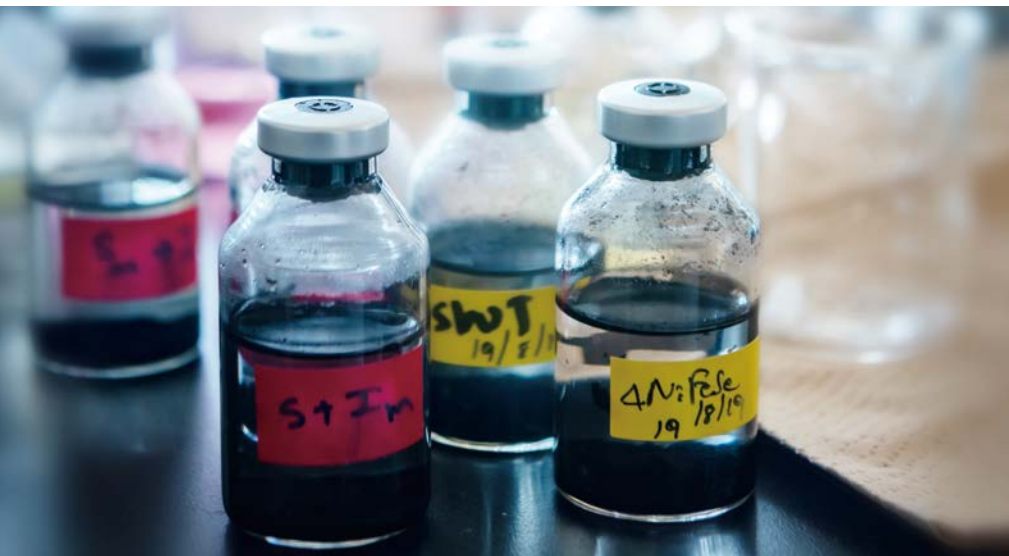
Sulfate-reducing bacteria in culture. Okamoto's group has been studying the impact of the bacteria on corrosion by changing the medium composition and manipulating bacterial genes. Iron sulfide (black rust) has been deposited at the bottom.
