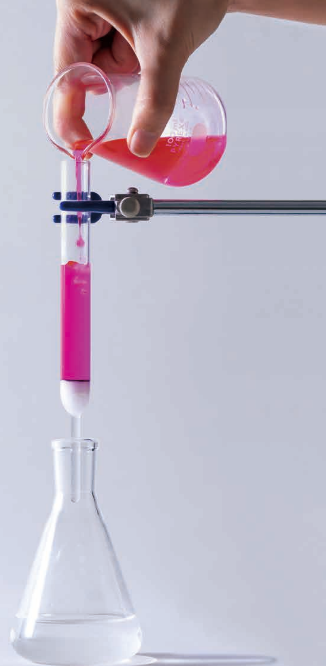
Dyed water becomes clear as it passes through a clay filter capable of removing only the pigment.
