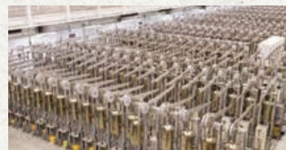
Array of creep testing machines at the NIMS Sengen Site facility
