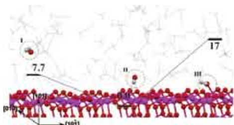
Fig. 2. Snapshot in the equilibrium trajectory of the TiO 2 anatase/acetonitrile interface with water molecule contamination. Characteristic hydrogen bond appears between the H 2 O molecule and TiO 2 surface.
