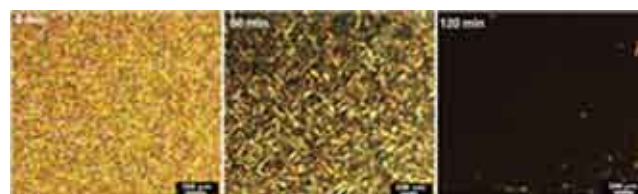
Fig. 2. Time-dependent magneto-optical response of orthorhombic liquid crystalline material at 420K under a 5T field. The optical images were taken with crossed-polarizers condition of the magneto-optical microscope.
