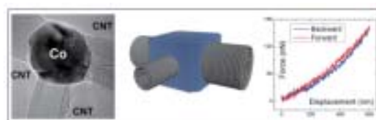
Fig. 3. HRTEM image (left), structural model (center) and force-displacement curves (right) recorded under tensile loading of plumbed multi-walled CNTs inside the AFM-TEM holder.
