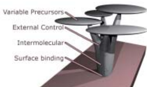
Figure 1. Depiction of the different factors that can be used to control nanoscale organic surface structure growth.
