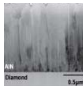
Fig. 2. XTEM of AlN on (111) diamond substrate.
