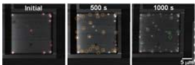
Fig. 3. EBIC images of an n-well cap before and after CVS at -3 V.
