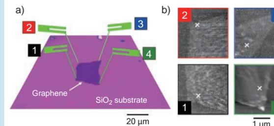
Fig. 2: Schematic diagram of a quadruple-probe atomic force microscope with tuning fork probes (TFP) enabling measurement of the properties of graphene with nanoscale precision. a) Schematic diagram of the four TFPs approaching a monolayer graphene flake measured by QP-AFM. The middle part shows the graphene flake, which is laid on a SiO<sub>2</sub> substrate. b) AFM images (3 × 3 μm<sup>2</sup> each) obtained at each corner of the graphene by using the four TFPs.
