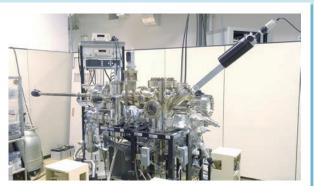
Fig. 1: The world-first double-probe scanning tunnelling microscope further improved at MANA.
