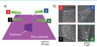
Fig. 2: Schematic diagram of a quadruple-probe atomic force microscope with tuning fork probes (TFP) enabling measurement of the properties of graphene with nanoscale precision. a) Schematic diagram of the four TFPs approaching a monolayer graphene flake measured by QP-AFM. The middle part shows the graphene flake, which is laid on a SiO<sub>2</sub> substrate. b) AFM images (3 x3  $\mu$ m<sup>2</sup> each) obtained at each corner of the graphene by using the four TFPs.
