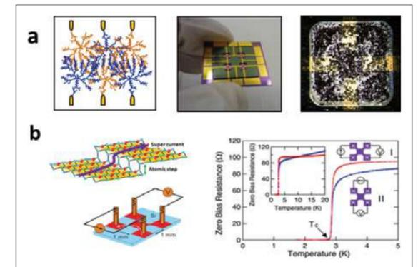
Fig. 1 a) Formation of a gigantic network of plastic devices to input signals, like synapses of the human neural network. b) Observation of surface superconductivity which is expected to enable novel qubits for quantum computing.
