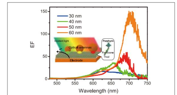
Size dependent photocurrent enhancement factor as a function of wavelength at optical antenna (gold nanoparticle) – molecule (porphyrin-ferrocene-thiol linked molecule) hybrid system on gold electrode.
