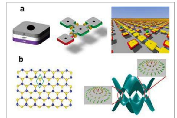
Fig. 2 a) Qubits which enable stable quantum calculation in which quantum interference can hardly be disturbed, and assemblies of those qubits. b) A 2-dimensional structure that enables a current to flow with zero electrical resistance.
