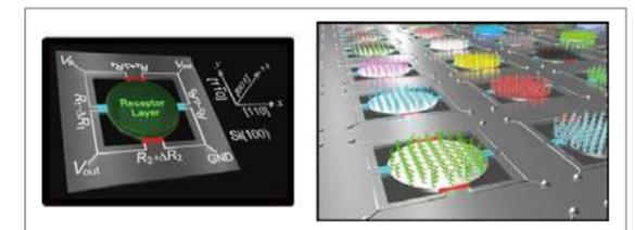
Fig. 3 New ultra-high sensitivity molecular sensor that enables super parallel analysis and identification of molecules in gases and liquids.
