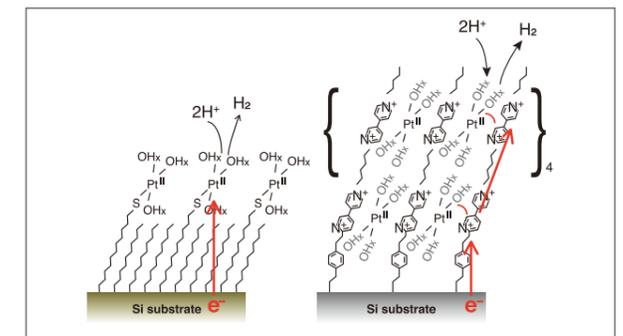
Surface confined molecular catalysts for photoelectrochemical hydrogen evolution at Si electrode.
