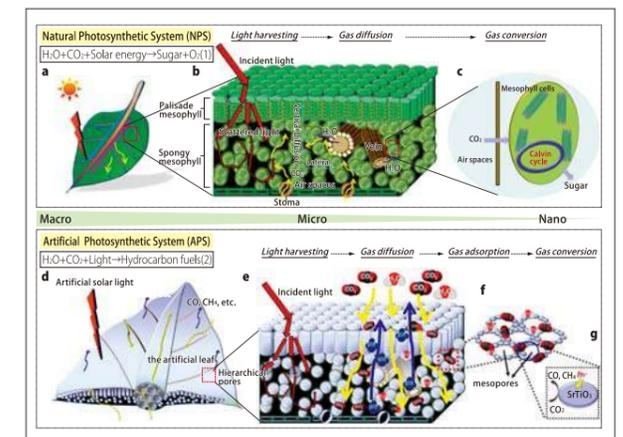
Fig. 1 Schematic illustration and comparison of the key processes in natural photosynthetic system (NPS) and artificial photosynthetic system (APS). Main processes are : light harvesting, gas adsorption, gas diffusion, and gas conversion.
