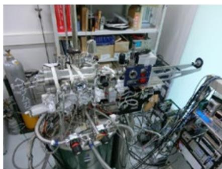
Fig. 2. Photo of the UHV-compatible cryostat for transport measurement in magnetic fields.
