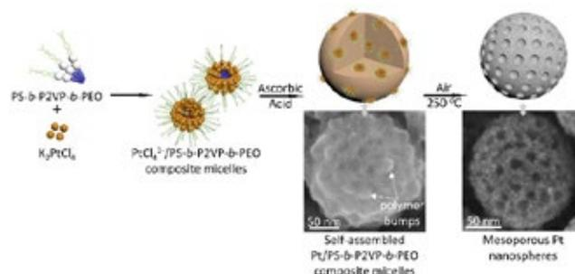
Fig. 1. Synthesis of mesoporous Pt nanospheres with tunable pore sizes prepared from polymeric micelle assembly.
