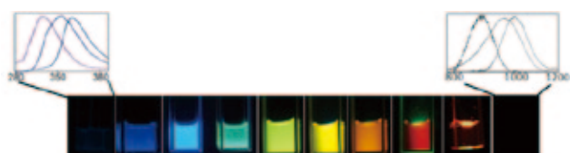
Fig. 1. Continuous tuning in the range between 300 nm and 1000 nm by the fine-structural control over silicon nanoparticles.
