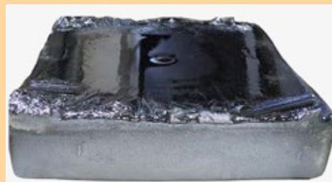
Photograph of the silicon ingot grown with the optimum conditions observed in the current study.
