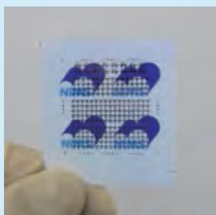
Fully printed organic thin film transistors (OTFTs) on a paper substrate.
