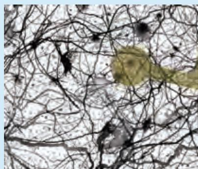
A look inside the ASN device reveals its highly interconnected architecture which comprises synaptic circuit elements at each point of contact between nanowires.
