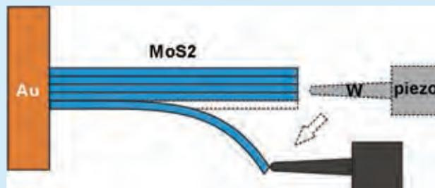
Nanomechanical cleavage of molybdenum disulphide atomic layers.
