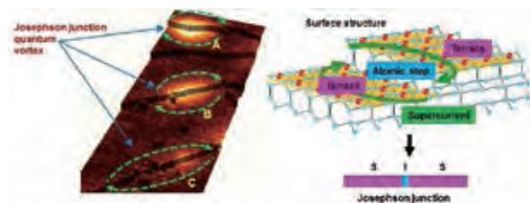
**Fig. 4-13:** (Right) Structure of the Si(111)-( $\sqrt{7} \times \sqrt{3}$ )-In surface having atomic steps each of which acts as a Josephson junction. (Left) Josephson junction quantum vortices observed by the scanning tunneling microscope (STM).
