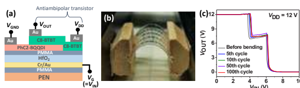
Fig. 1. (a) Device structure (b) Flexible MVL on bending test setup (c) Voltage transfer curves, showing excellent mechanical stability.
