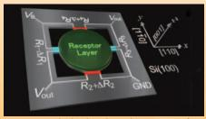
Figure 2. Newly developed Membrane-type Surface stress Sensor (MSS). The surface stress induced by an adsorption of analytes on the center membrane is efficiently detected by the piezoresistors embedded at the four peripheral beams.
