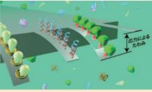
Figure 1. Schematic image of the measurement of various analytes ranging from gaseous to biological molecules using an array of microcantilevers. The deflection induced by an adsorption of analyte molecules is measured as a signal.
