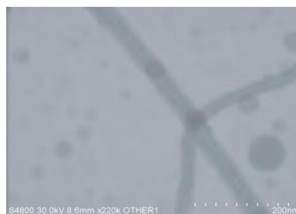
Figure 2. STEM image of polymer /MWNT composite.
