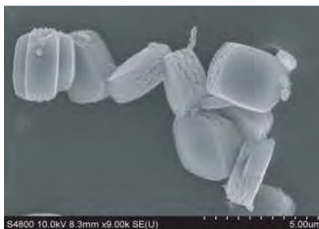
Fig 1 (right): HR-FESEM image of crystalline mesoporous titano silicates.
