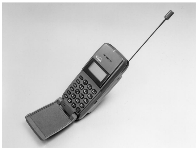
Fig. 23. Superelastic antenna for a cellular phone. (Courtesy of Fujitsu Corp.)
