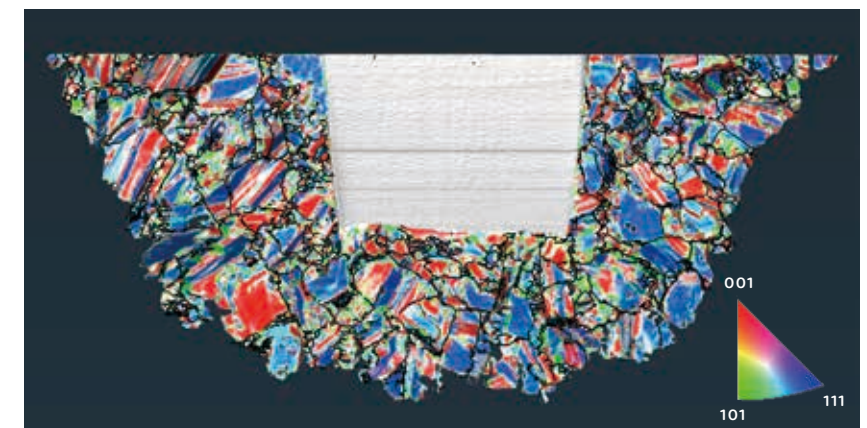
Image showing the orientations of crystals around the traces of crack growth. A majority of cracks were found to propagate along the (111) crystalline plane known as the slip plane (shown in blue).
