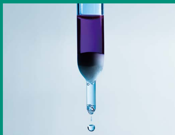
The clay filter placed in the pipette adsorbs only the pigment in the liquid material.
