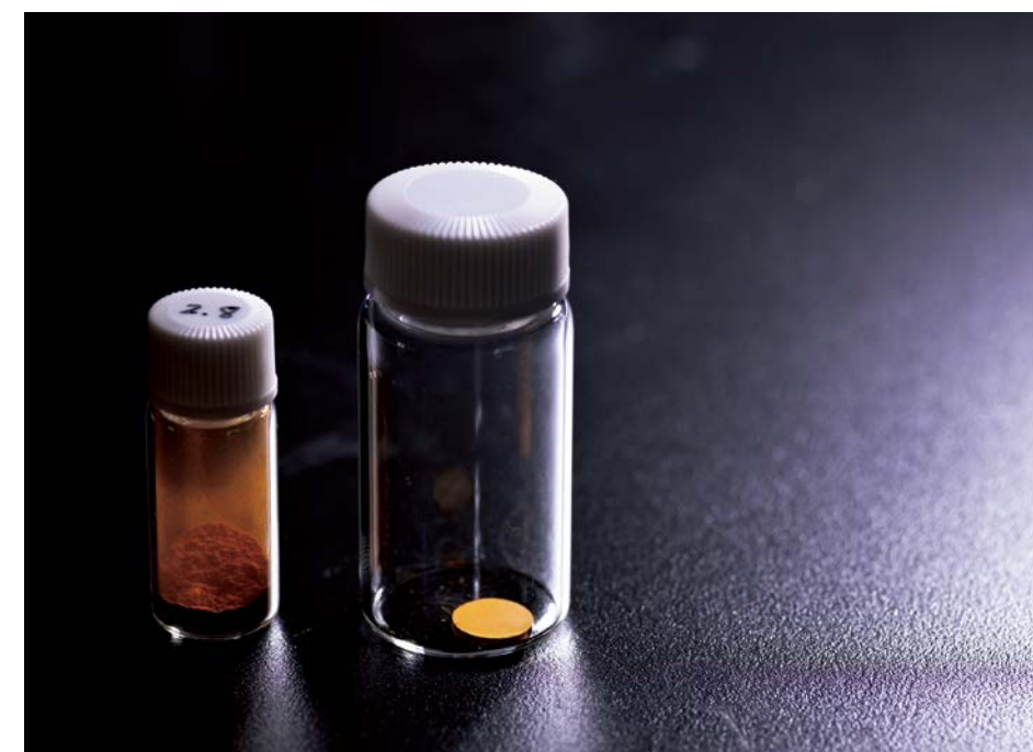
Lanthanum oxyhydride powder (left) and the product formed after it was compacted and sintered (right). Lanthanum oxyhydride can be synthesized by mixing lanthanum oxide with lanthanum hydride and heating the mixture.
