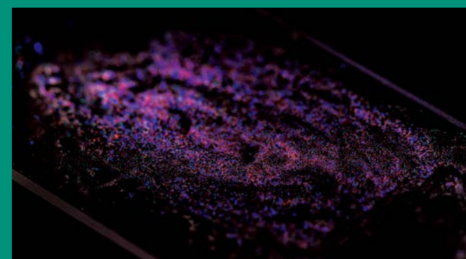
A phosphor developed for use in an LED light source emits visible light when subjected to ultraviolet irradiation.
