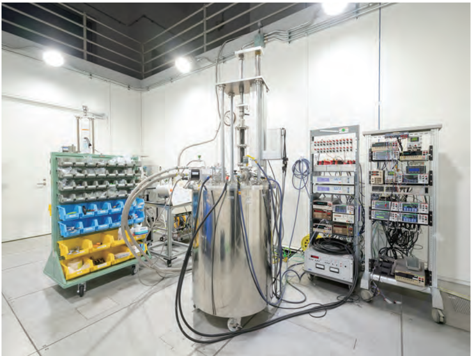
Prototype magnetic refrigerator capable of liquefying hydrogen
