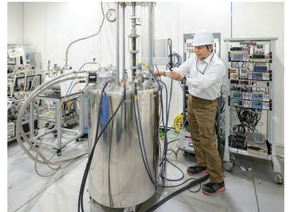
Koji Kamiya (Group Leader of Magnetic Refrigeration System Group) operating a magnetic refrigeration prototype for hydrogen liquefaction
