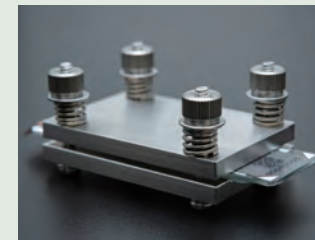
High energy density lithium-air battery cell equipped with a porous carbon cathode developed by NIMS
