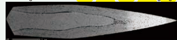
Backscattered electron SEM image of a cross-section of a Japanese sword. Martensite can be seen at the tip of the blade material. (Photos provided by Mr. Kazunori Tsukamoto and Dr. Takashi Kimura, JEOL Ltd.)
