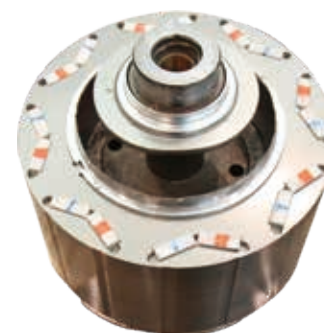
Electric vehicle motor equipped with dysprosium-free magnets
