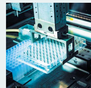
Pipetting unit Each well receives an electrolyte with a different composition. After the pipetting process is completed, the multi-well microplate is transferred to the electrode unit by the robot arm.
