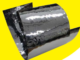
Vanadium (V) alloy foil enabling separation and purification of hydrogen developed by Nishimura. The rate of hydrogen passing through the foil can be increased by reducing the thickness of the foil.
