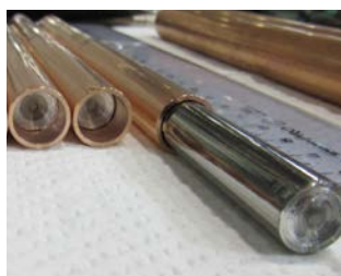
Figure 3. Jelly roll-processed billets fabricated at the NIMS facility. The billets are produced by wrapping Nb and Al foil of 0.1 mm and 0.03 mm in thickness, respectively, around a Nb core bar. To produce a multicore wire, a billet is processed into a thin wire by inserting it into a copper tube and pushing it out using a hydrostatic extrusion process. Hundreds of thin wires are then bundled together to form a multicore wire.
