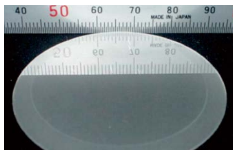
Oshima succeeded in growing single-crystal films of approximately 2 inches in diameter.
