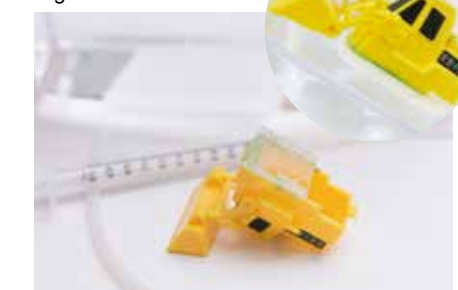
A polymer material was attached to the bottom of a bulldozer model to mimic the mechanism of tarsal hairs of the leaf beetle. When bubbles are applied to the material underwater using a syringe, so that the material's surface catches the bubbles, the material tightly adheres to the glass surface.
