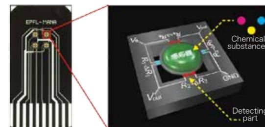
An MSS chip (left) and a magnified inset showing an MSS element (right). The distance between each MSS element is about 1 mm. When molecules adsorb to a receptor layer coated on the circular center membrane, surface stress is induced, causing electrical signals through the electric resistance changes of the piezoresistors embedded in the four supporting bridges.
