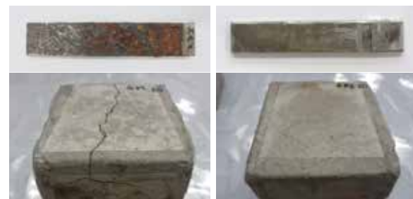
Appearance of conventional carbon steel (left) and newly developed corrosion-resistant steel (right) after used as concrete reinforcing steel during two-year exposure tests at the Irapu Ohashi Bridge. The concrete block containing carbon steel cracked due to expansion caused by steel corrosion, while the block containing corrosion-resistant steel did not.
