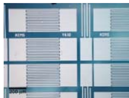
Fig. 1 Diamond UV sensor fabricated on the hydrogen-terminated surface.
