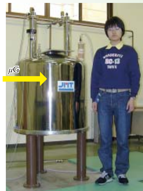
Fig. Superconducting magnet used to obtain a microgravity environment.
