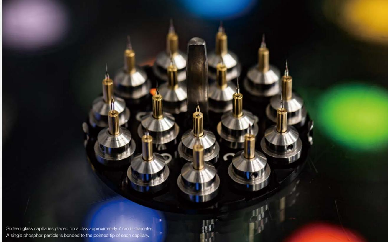
Sixteen glass capillaries placed on a disk approximately 7 cm in diameter. A single phosphor particle is bonded to the pointed tip of each capillary.
