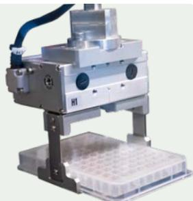
Robotic arm carrying a microplate based electrochemical cells
