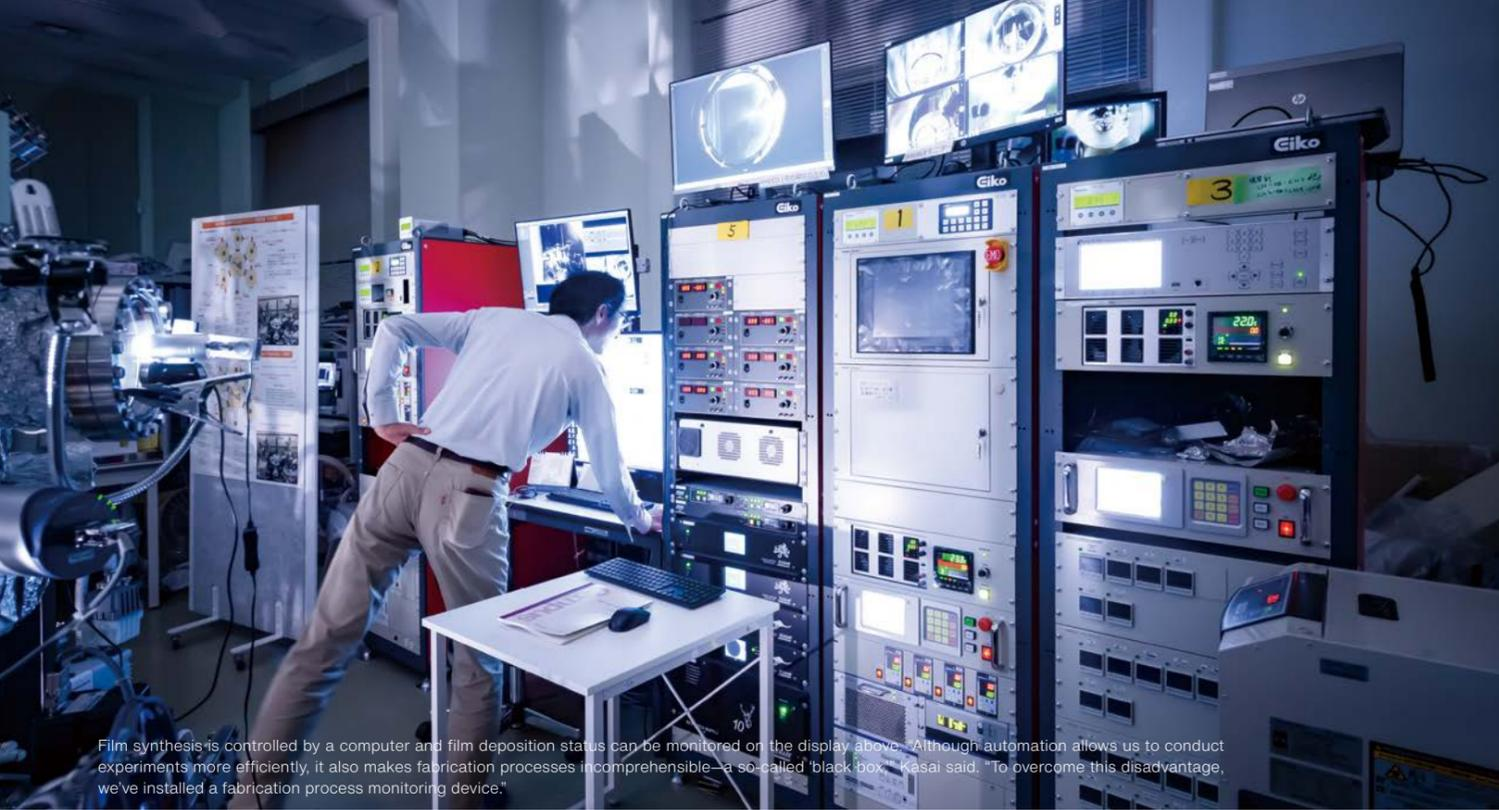
Film synthesis is controlled by a computer and film deposition status can be monitored on the display above. Although automation allows us to conduct experiments more efficiently, it also makes fabrication processes incomprehensible—a so-called “black box,” Kasai said. To overcome this disadvantage, we’ve installed a fabrication process monitoring device.
