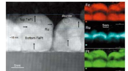
Figure 2. Transmission electron microscope (TEM) image of a three-dimensional recording medium
