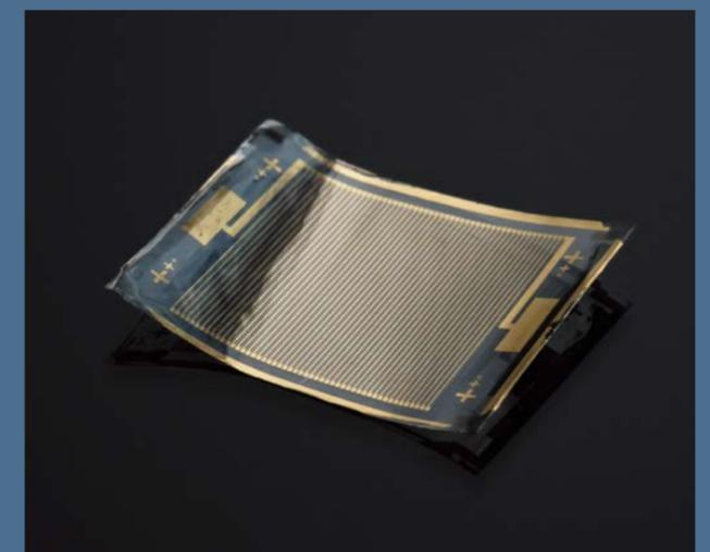
Bendable, flexible thermal flux sensor (see p. 10)
