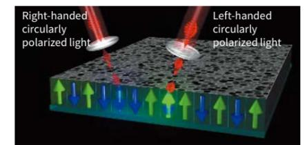
Figure 4. Conceptual diagram illustrating how magnetization reversal can be induced using circularly polarized light
