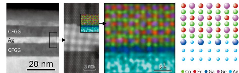
Figure 1. Interface structure and elemental distribution of a CPP-GMR device using half-metallic Heusler alloy as ferromagnetic layers.
