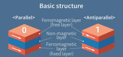
\*The non-magnetic layer of a tunnel magnetoresistance (TMR) device is made of an insulator, while that of a giant magnetoresistance (GMR) device is made of a metal.
