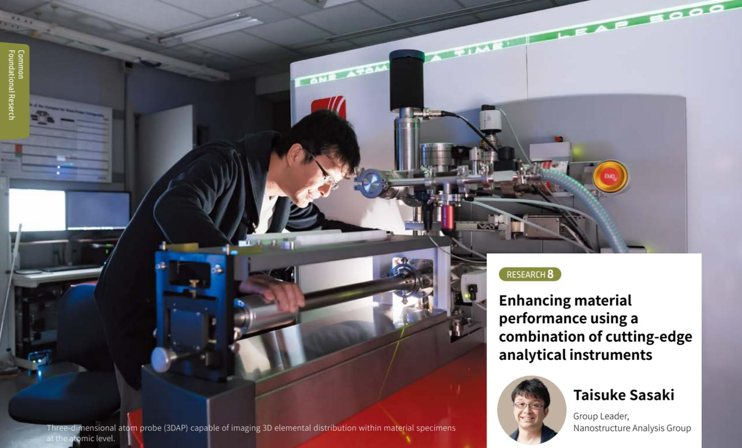
Three-dimensional atom probe (3DAP) capable of imaging 3D elemental distribution within material specimens at the atomic level.
