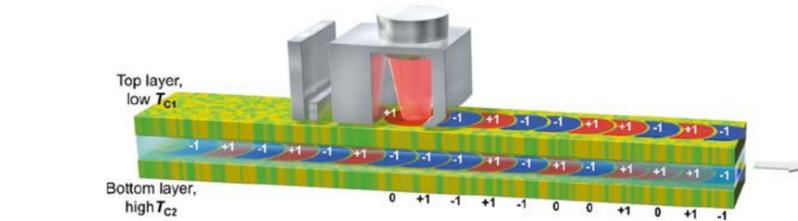
Figure 1. Conceptual diagram illustrating multi-level magnetic recording
