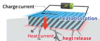
Figure. Example of a hybrid material functioning as a thermoelectric permanent magnet
