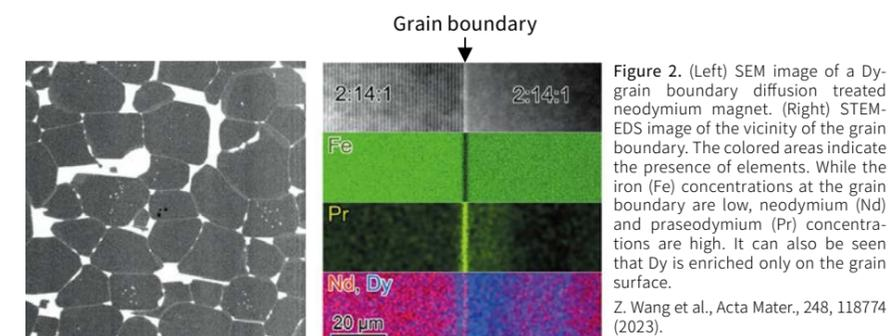
Figure 2. (Left) SEM image of a Dy-grain boundary diffusion treated neodymium magnet. (Right) STEM-EDS image of the vicinity of the grain boundary. The colored areas indicate the presence of elements. While the iron (Fe) concentrations at the grain boundary are low, neodymium (Nd) and praseodymium (Pr) concentrations are high. It can also be seen that Dy is enriched only on the grain surface.
