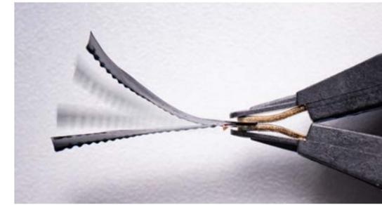
**Voltage application causes the film to flex**
