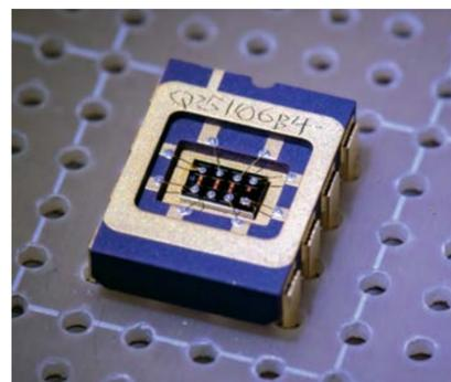
**Prototype infrared detector equipped with striped optical antennae**
