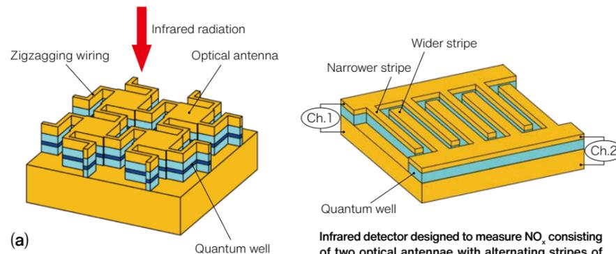
**Infrared detector designed to measure NO<sub>x</sub> consisting of two optical antennae with alternating stripes of different widths**
