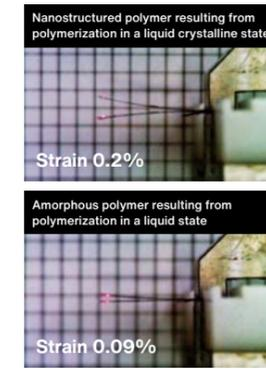
**Comparison of displacement between films with and without the columnar structure**
