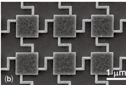
**Metamaterial infrared detector developed by Miyazaki**
